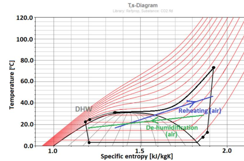
Figure 5.5: Heat pump assisted drier with R744 for drying temperature of 45°C.
