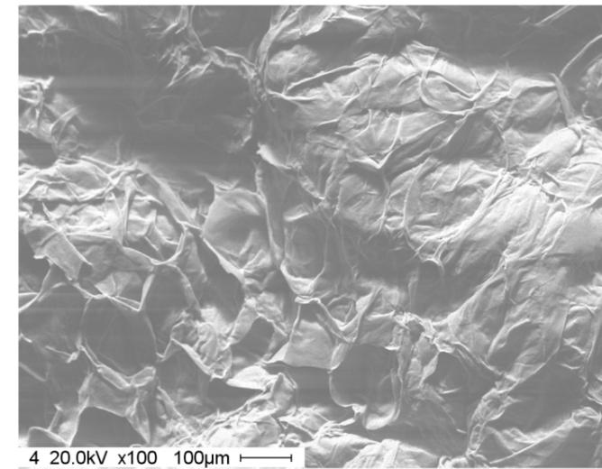
Figure 1.1.13: Visible surface of sample 1, magnified 100 times,  $X_0 = 8.3$  gw/gd
