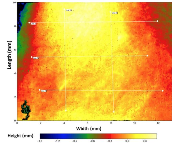
Figure 1.1.9: Topographic mapping of the surface of sample 1 after drying,  $X_0=8.3$  gw/gdm
