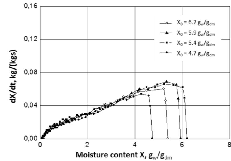
Figure 1.1.6: Drying rates for different initial moisture contents as a function of moisture content, drying conditions like in Figures 3
