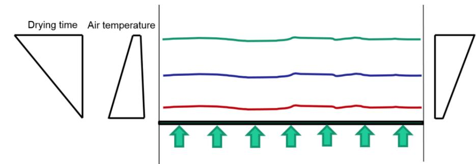
Figure 4.7: Impact of bulk height/weight on temperature decrease, air humidity increase and duration of drying process
