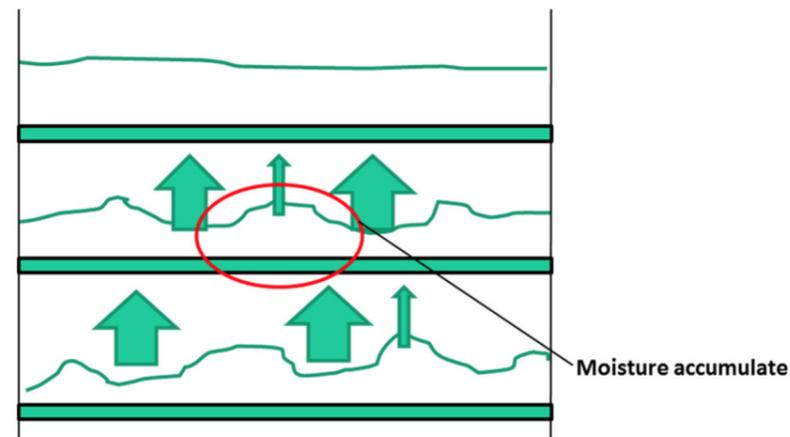
Figure 4.6: Produce distribution and air flow distribution in a multi stage dryer (Sturm, 2017b)
