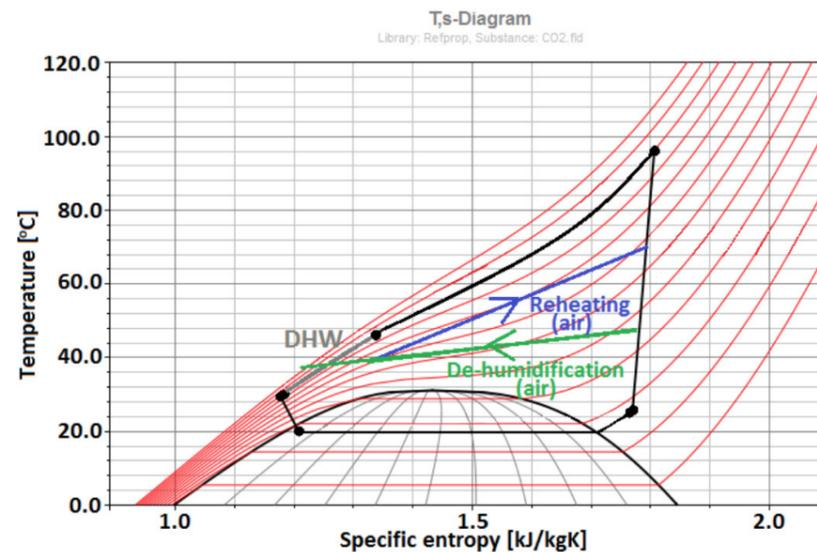
Figure 5.7: Heat pump assisted drier with R744 for drying temperature of 70°C.
