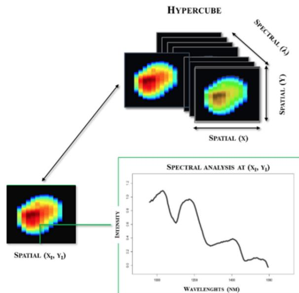
Figure 6.3: Schematic representation of a hypercube (Raponi et al., 2017)
