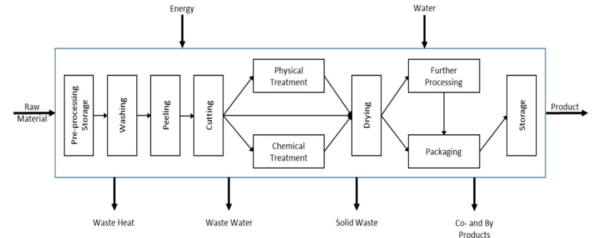
Figure 4.1: Overview of processing steps in the production of dried agricultural goods (Sturm, 2017)
