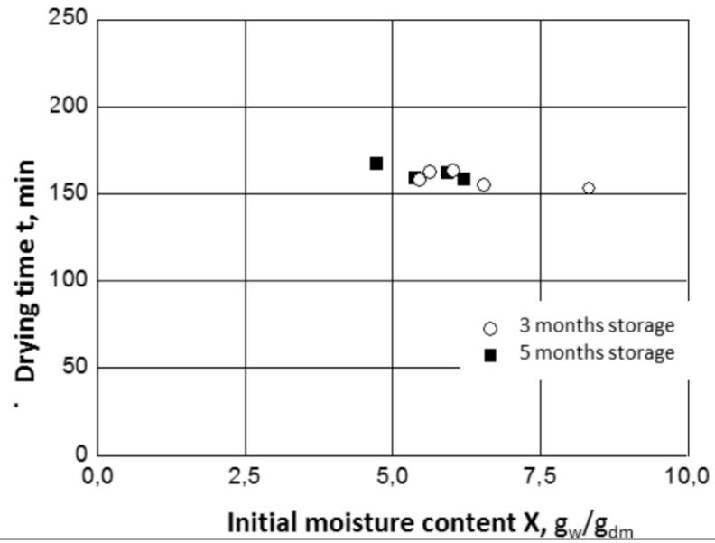
Figure 1.1.5 Drying time of apple slices down to a final moisture content of 0.13 gw/gdm related to initial moisture content. Drying conditions like in Figure 3
