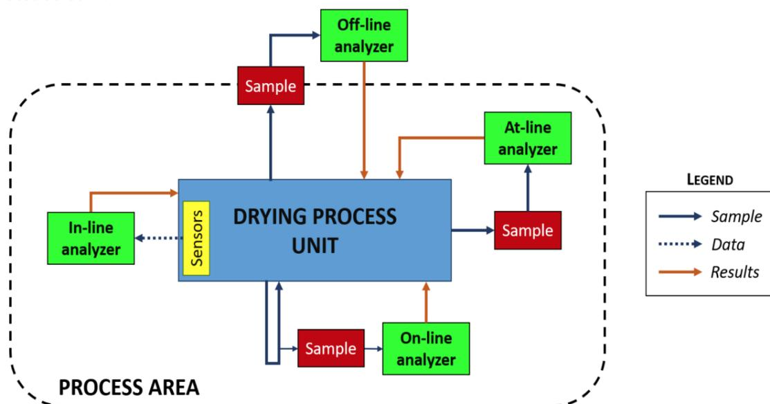
Figure 6.5: Schematic of the differences among off-line, at-line, on-line and in-line measurement techniques (Raponi et al., 2017)
