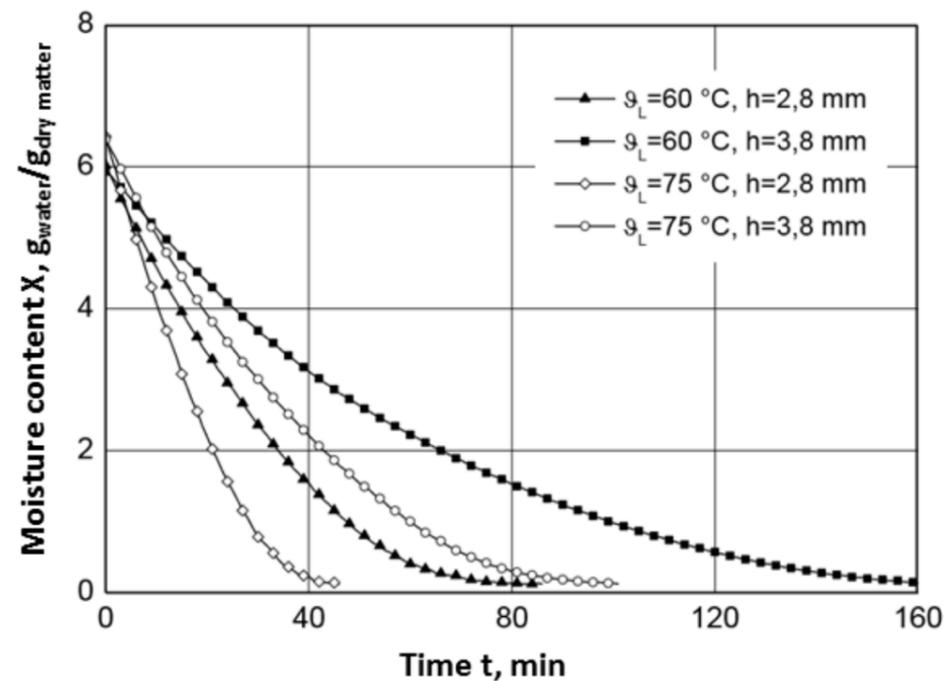
Figure 4.2: Drying behaviour depending on slice thickness and temperature (adapted from Sturm, 2010)
