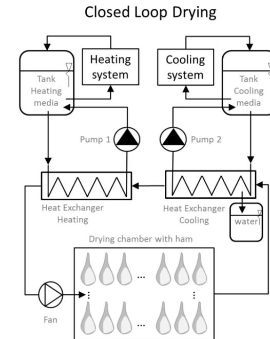
Figure 5.2: Industrial closed loop drying, which requires cooling and heating of the circulated drying air in order to remove the evaporated water.
