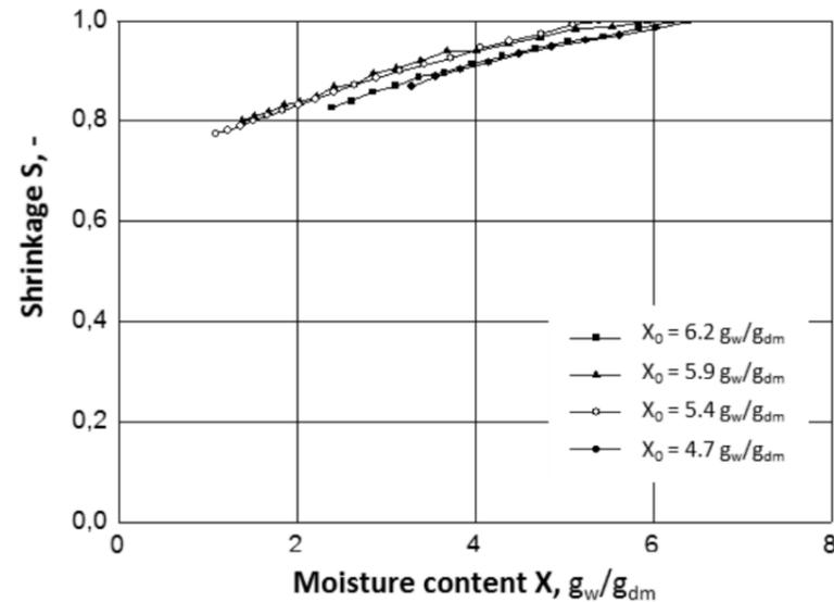
Figure 1.1.8: Shrinkage  $S$  for different initial moisture contents  $X_0$  as a function of moisture content, drying conditions like in Figure 3
