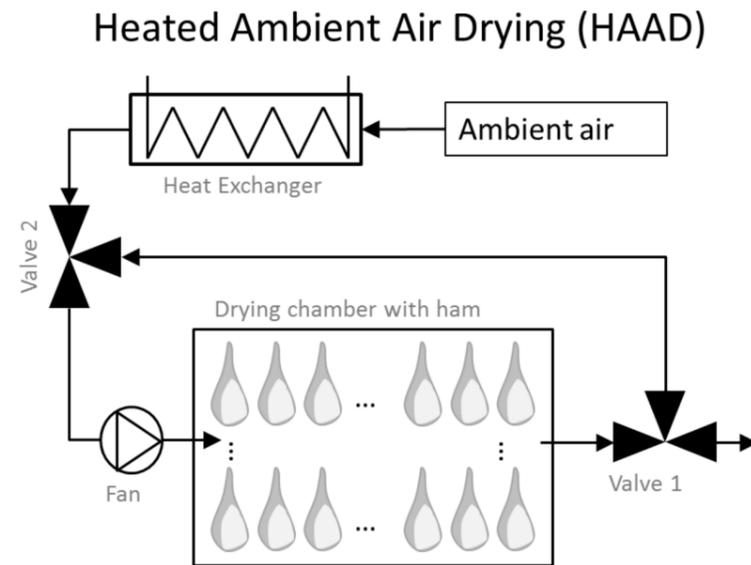
Figure 5.1: Sketch of a heated ambient air drier which is commonly used in the industry.
