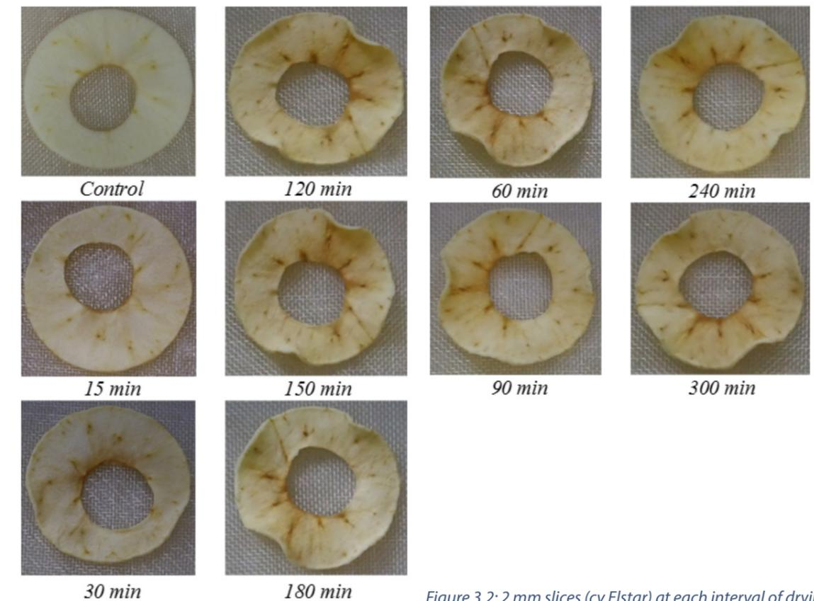
Figure 3.2: 2 mm slices (cv.Elstar) at each interval of drying period at 70 °C
