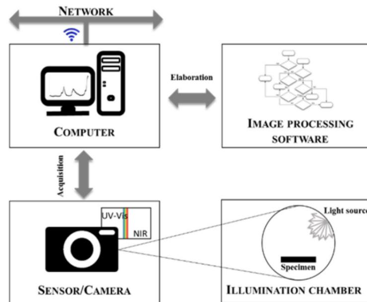
Figure 6.1: Element of a computer vision system (Raponi et al., 2017)
