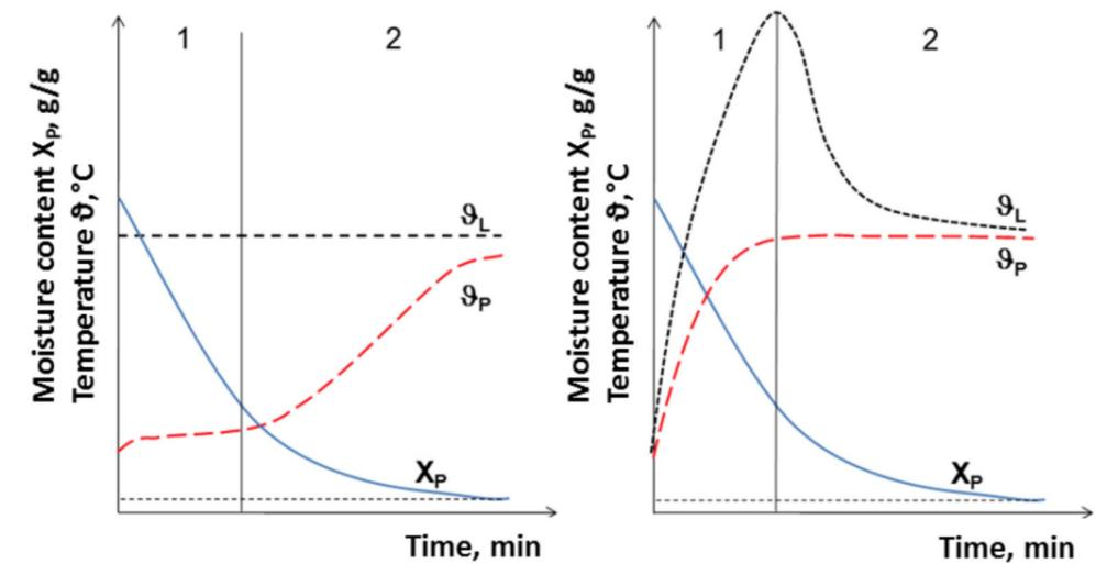
Figure 4.10: Temperature development during air temperature and product temperature controlled drying (Sturm, 2010)
